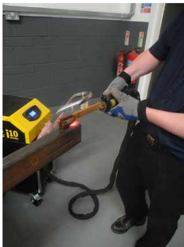
Figure 6.6 — The 4 kW (left) and 10 kW (right) induction heaters being used to heat metal components in the repair shop. In these cases the transformer is housed in a separate power unit (left of pictures), with electrical and coolant supply cables connecting the power unit to the heating element (being held by worker in each case). These contrast with the much simpler 1 kW induction heater shown in Figure 6.3
