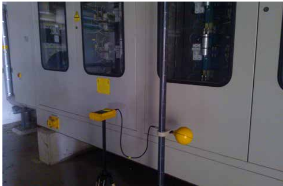
Figure 3.6 — Measurements being made near a thyristor rectifier
