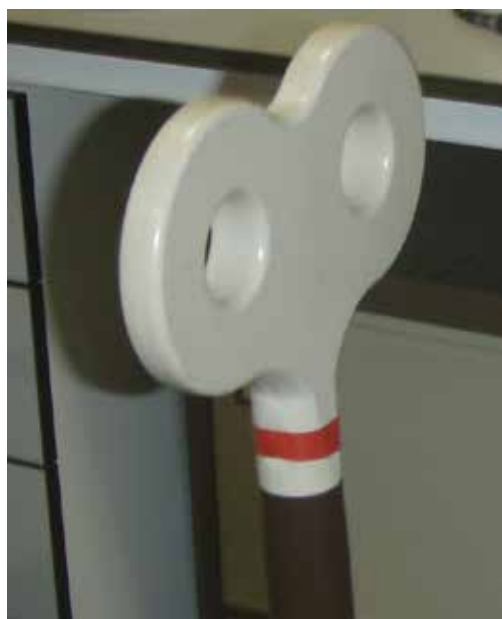
Figure 4.2 — ‘Figure-of-eight’ TMS coil
