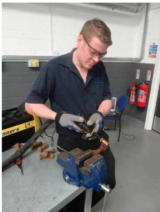
Figure 6.6 — The 4 kW (left) and 10 kW (right) induction heaters being used to heat metal components in the repair shop. In these cases the transformer is housed in a separate power unit (left of pictures), with electrical and coolant supply cables connecting the power unit to the heating element (being held by worker in each case). These contrast with the much simpler 1 kW induction heater shown in Figure 6.3
